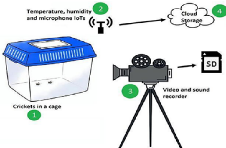
Figure 6: ICIPE experimental set up used to study cricket behaviour to improve cricket farming.
